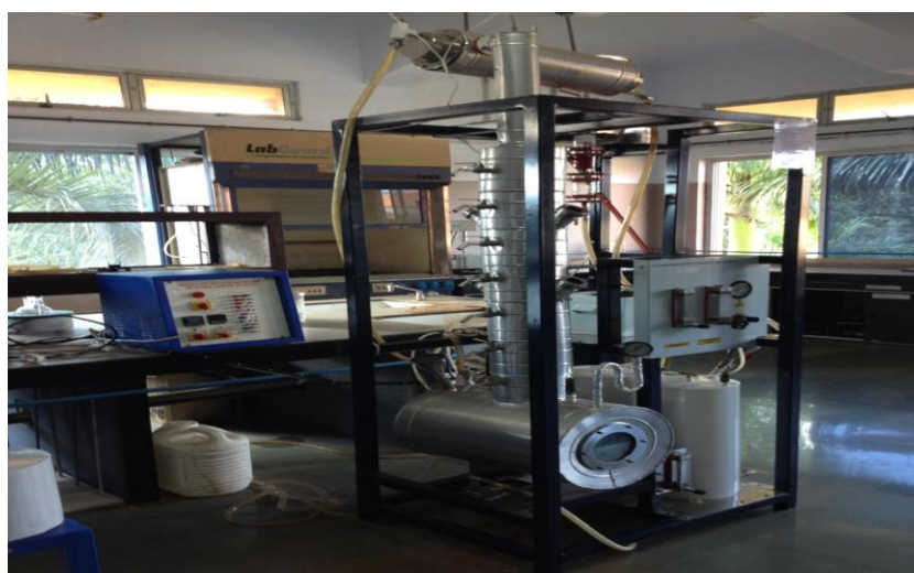
Figure 12:- Bubble Cap Distillation Column
