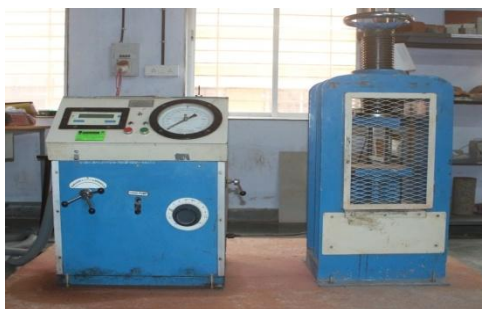
Compression Testing Machine in Concrete Technology Lab
