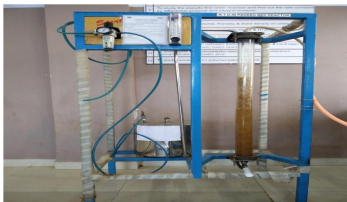
Figure 17:- ResidenceTime Distribution of Packed Bed Reactor
