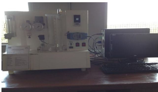
Figure 20:- Level Controller Trainer
