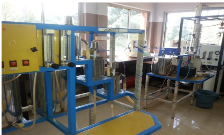
Figure 16:- CascadeContinuous Stirred Tank Reactor.
